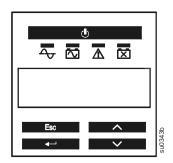
Reset the Battery Install Date for the internal UPS battery.
