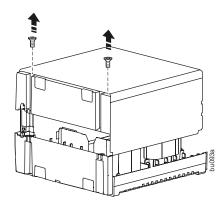
3 Detach the red and black wires from the battery. Remove the old battery and replace with new battery. Reconnect the battery wires, red to the + and black to the -. Reassemble the unit.
