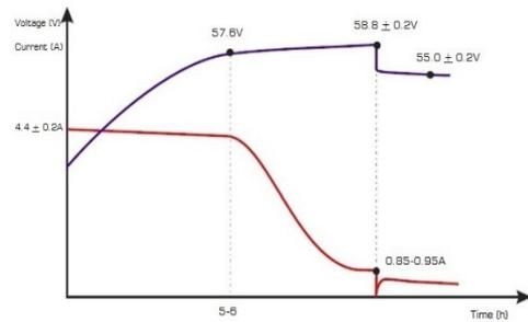
**Phase 1:** The Max. charge current is 4.4A, and the charge voltage is gradually risen up to 57.6V;
