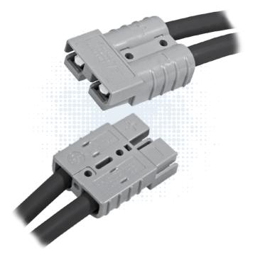
Based off the design pioneered by Anderson in 1953, APP®'s two pole SB® connectors set the standard for DC power distribution and battery connections. SB®50 connectors feature a one piece plastic housing using stainless steel springs to hold low resistance contacts in place. Wires sizes from #16 (1.5 mm<sup>2</sup>) to #6 (13.3 mm<sup>2</sup>) are held in the smallest of the SB® series housings.
